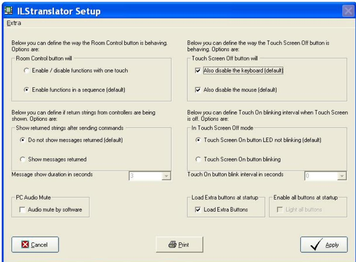
Under Room Control button you can select whether all functions will be enabled/disabled with one touch or in a sequence.
