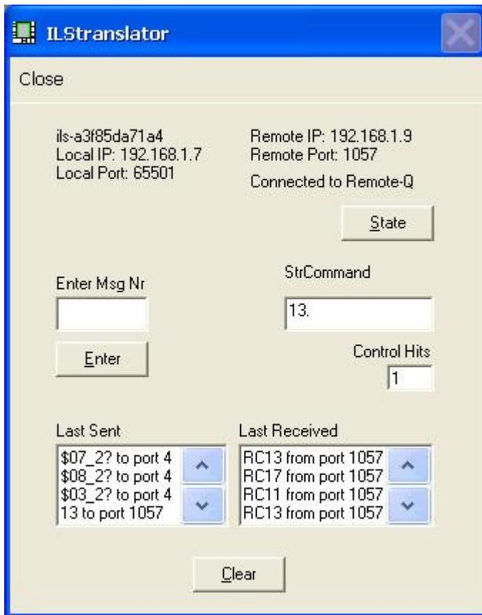
Note: By 'showing' the ILTranslator Main form you can also verify the connection status to external control programs. In this case, ILTranslator is connected to Remote-Q over TCP/IP. The State button in this form will show the state of the connection, with the menu Close command you can close the connection. The ILTranslator listening port, via ILS22Setup, was set to 65501.
