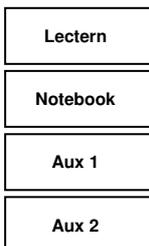
This group of keys is intended to select the output source, whether the Lectern System, an external connected notebook PC or Auxiliary devices such as DVD player or other devices. Lectern is used by default. If an intelligent external switch controller is connected (via RS232), command strings can be send to the controller. In the standard version, these keys are NOT defined, as they are dependent on manufacturer and model.
