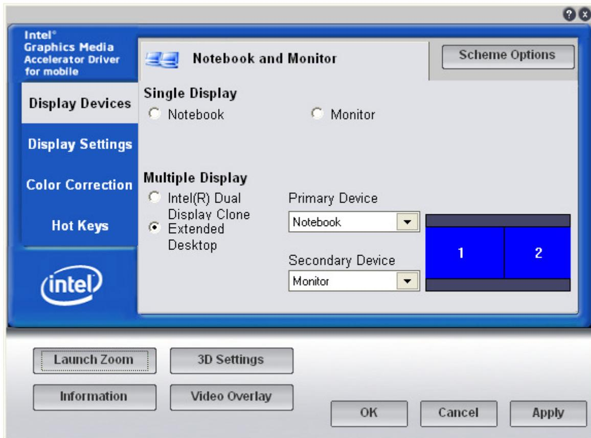
Hit Display Settings if you want to alter the ILS22 resolution/rotation (Notebook). Default value is 1680 \* 1050, 180 degrees rotated. Hit Monitor if you want to adapt the external monitor/projector resolution/rotation. In this case resolution settings are for Extended Desktop (Span).
