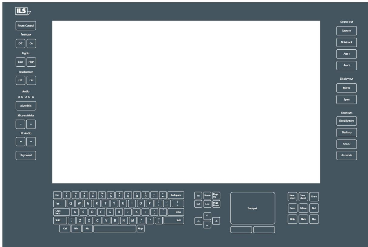
Where as the inner-side of the glass-plate functions as touch-screen for the LCD and the operating system, the outer sides (left, bottom and top) contain engraved headers and buttons for additional functions and the integrated keyboard. These functions are available to the presenter if they are visible with the backlight turned on.
