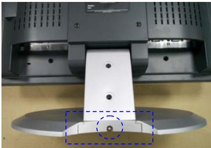
16. Paste rubber on screw hole of stand.
