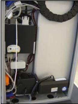
The optional PC is located on the left half of the base column. It is fastened to the base of the console vertically via a special fixture.
