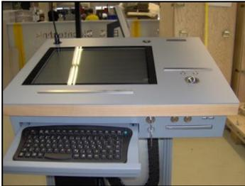
The touch screen has been inserted surface-flush in the vertical column.
