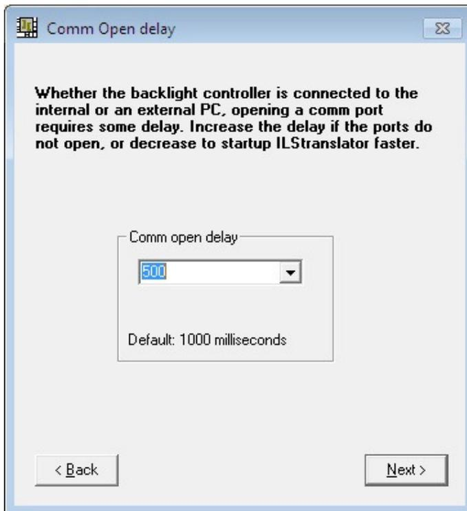
In the above form you can specify the number of milliseconds to wait before the comm. port gets active after opening it. If the internal PC is used, comm. ports may open successfully in just 250 milliseconds. With an external PC it may take longer. This entry allows to fine tune the system and has an impact on the ILStranlator start-up time.
