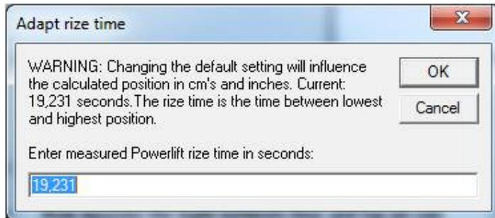
Once the calibration has been performed, you can move the pedestal up or down into a desired default position:
