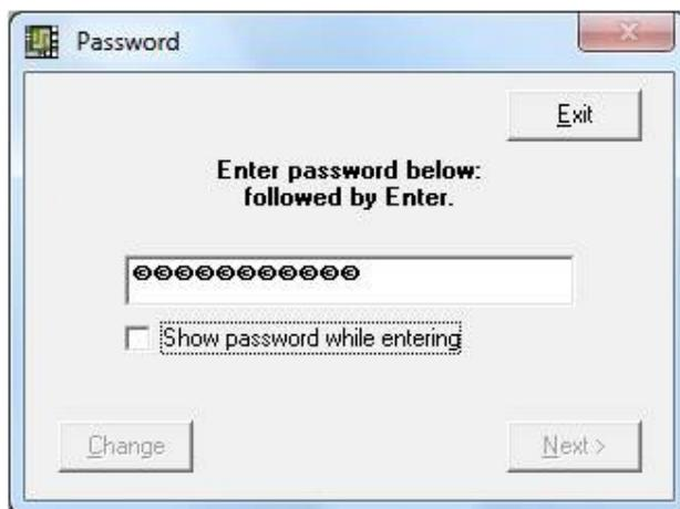
After entering the password (do not forget the Enter button in the end), the Next button and Change buttons are enabled. Change allows to make a new password.
