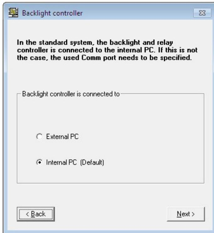
When the ILS22 is delivered in a standard setup, an internal PC is used to control the system and the backlight and relays controller. The internal PC has 5 serial comm. ports, of which COM4 is used to communicate with the backlight controller (see above scheme). In situations where an external PC is used, ILStranlator needs to know to which comm. port.
