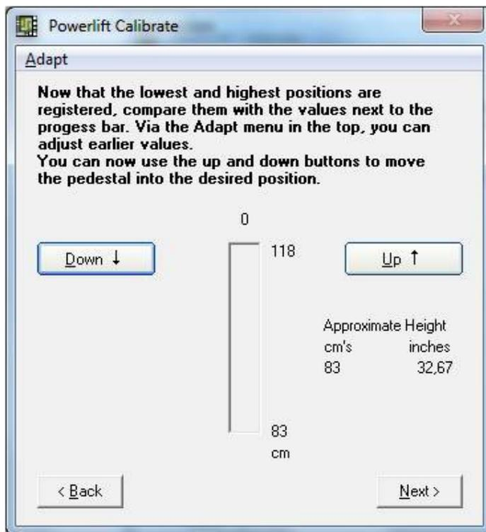
Hit the Down or Up buttons to elevate the pedestal into a required default position. The approximate height values will be adjusted accordingly.
