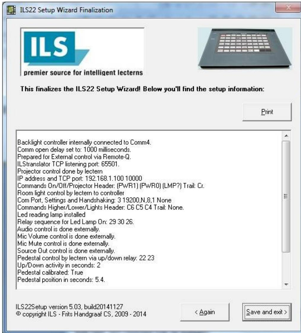
If you want to change the system setup, press on the Again button and Continue button in the startup window.
