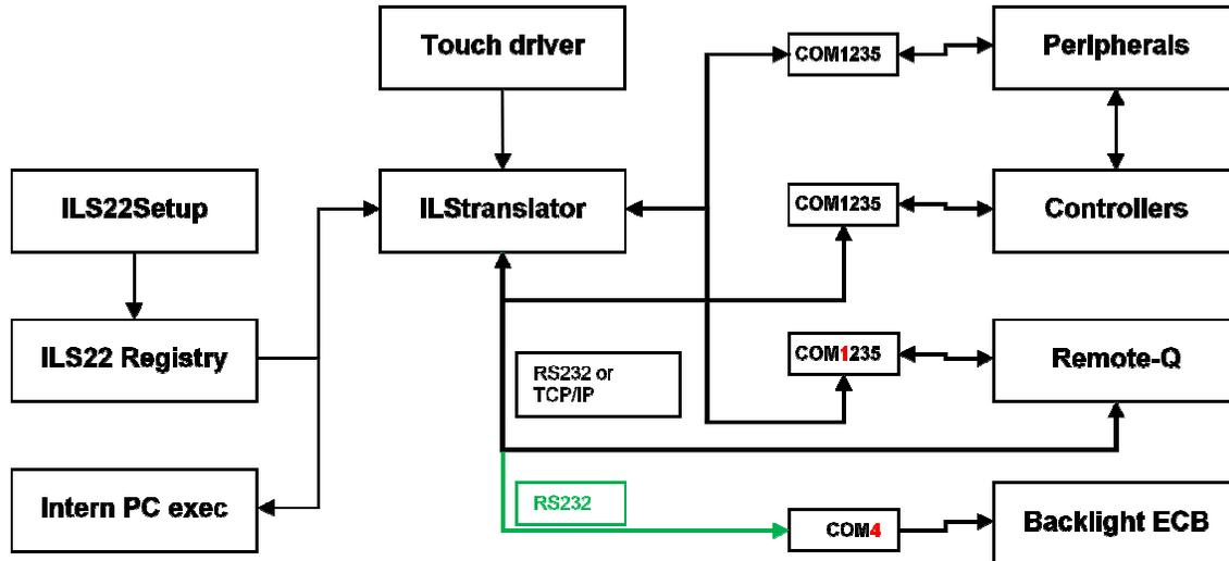
Note: All attached peripherals and/or controllers can be connected either via RS232 or TCP/IP. The Backlight and Relay controller can only be reached over RS232. COM4 is reserved for that purpose. If you want to connect to Remote-Q over RS232, COM1 by default is reserved for that purpose.
