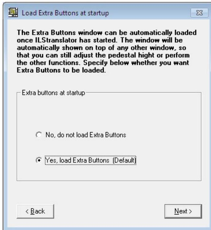
When loaded, you can adjust pedestal height, change ILStranlator settings (not ILS22Setup settings), show the Main window (which displays sent commands, received commands, connection status to Remote-Q) and can serve as a debug tool. In the Extra Buttons window you can also end ILStranlator from running, or hide the Extra Buttons window.
