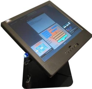
**Resistive touch** PC integrated 3GHz Dual Core power. DVD, 4 USB, 2 Firewire, SD card reader, PC audio I/O, VGA out, 1 serial port, LAN, PS2 keyboard/mouse ports **on solid lectern oriented table top stand.**
