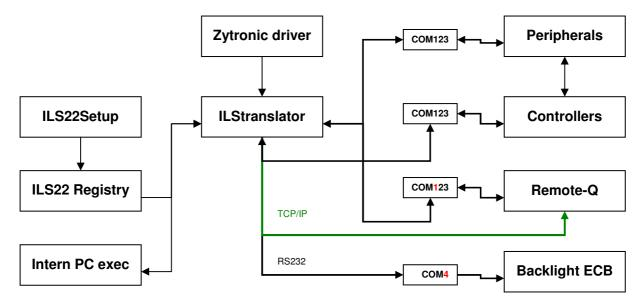
Via Com1, Com2 or Com3, ILStranslator can directly control projectors or other peripherals, or pass control over to intelligent attached controllers, which in turn can control the environment. Use the ILS22Setup Wizard to define the system setup.
