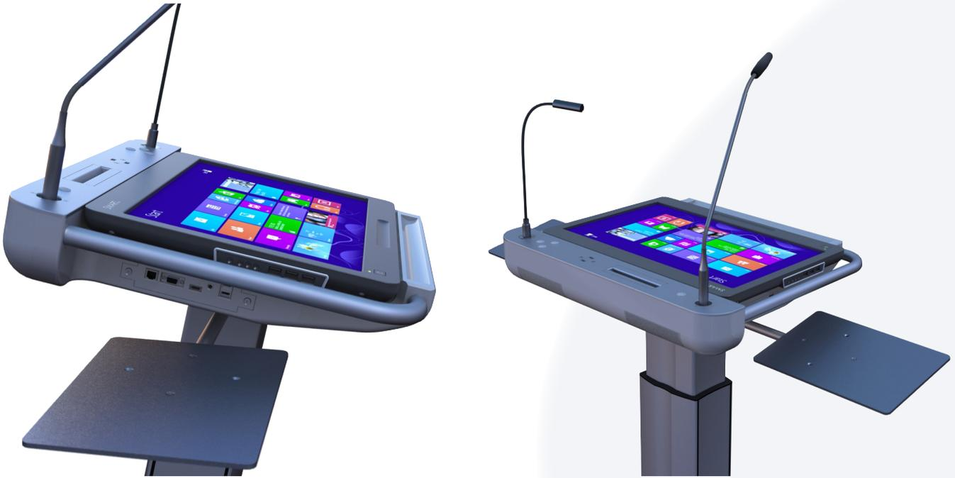
The new Synergy ST uses a Universal Mounting System with a VESA mount on top that allows for the use of a SMART SP254. This pen and touch monitor creates a very versatile lectern for both presentation and annotations. The Synergy ST requires a PC to control the screen, this PC can be placed remotely, either through a wall or floorbox, or inside the base. Alternatively, there is space inside the UMS for a Giada i57 micropc (i5).
