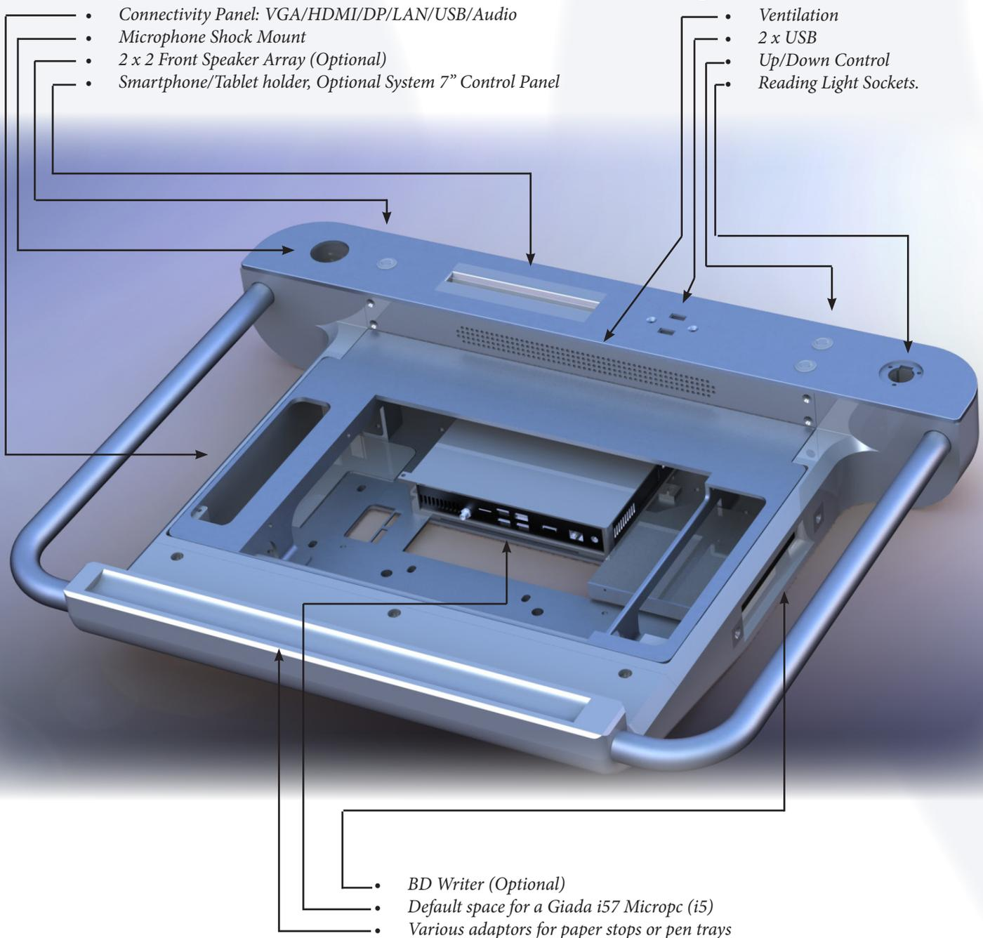
The new Synergy Platform has been redesigned from the ground up to be a fully integrated but modular system with space for many different options and solutions.
